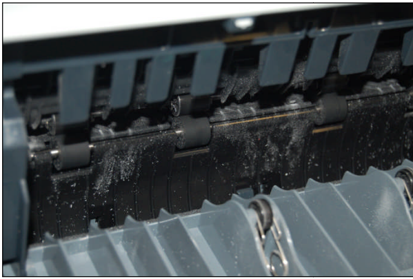
Left: Paper Dust Accumulation – Tested abrasive, large-particle filler papers that don't meet the ColorLok® quality standard
